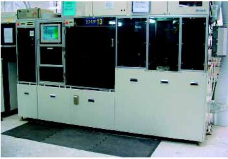
**Figure 1:** An automated DVD bonder, at the WAMo facility in Pennsylvania uses pulsed curing.
