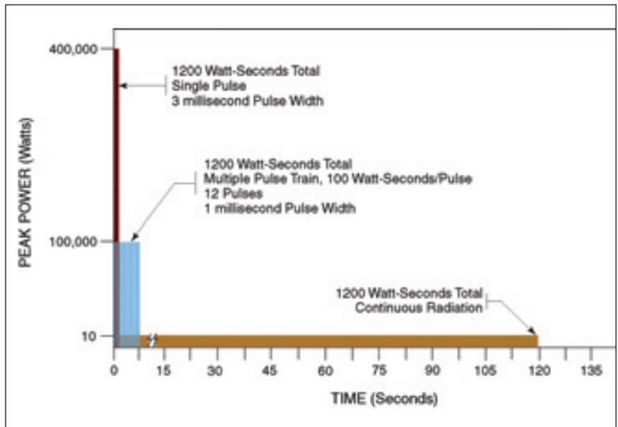
Figure 5. Pulsed UV Provides Cooling Zones Between Pulses
