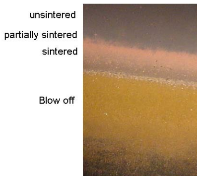
Figure 6: Copper Nanoparticle on Kapton with different intensity of light showing regions that are unsintered, partially sintered, sintered and evaporated
