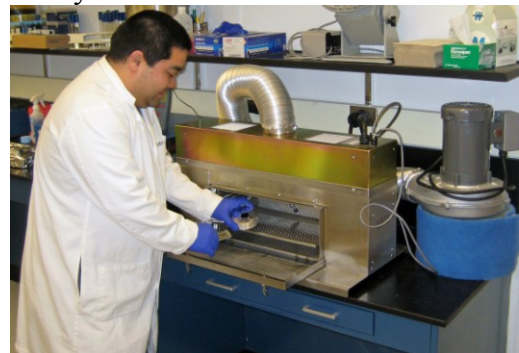
Figure 1: Aaron Uesugi setting up for fluence measurements using RS-3000C Steri Pulse System from Xenon Corporation (Woburn, MA).
