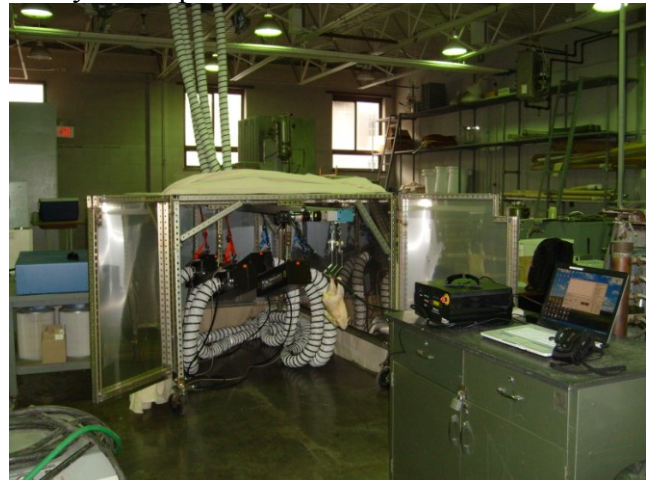
Figure 2. Pilot-scale continuous pulsed UV-light system for decontamination of chicken carcasses.
