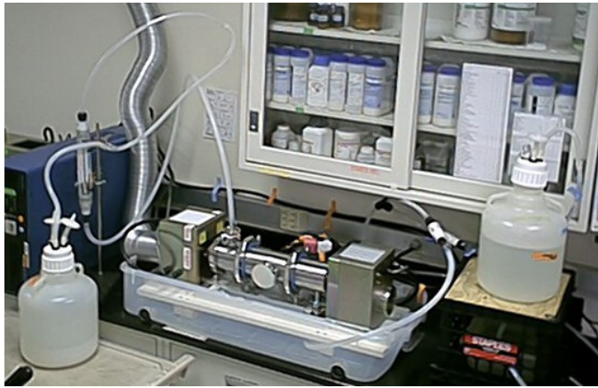
Figure 1. Flow-through pulsed UV light chamber (Steripulse®-XL 4000, Xenon Corp., Xenon Corp., Wilmington, MA).
